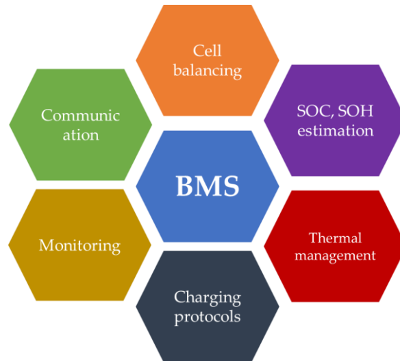
Figure 17. BMS main functionalities.
