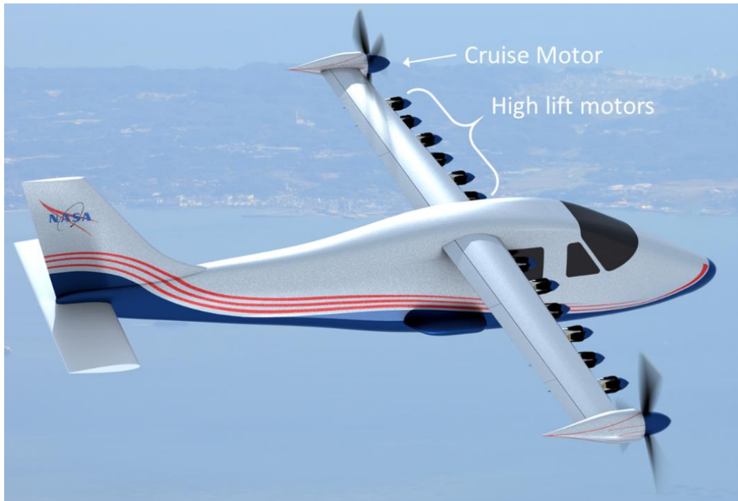
Figure 3. Concept of NASA's X-57 Maxwell aircraft with distributed electric propulsion [2]
