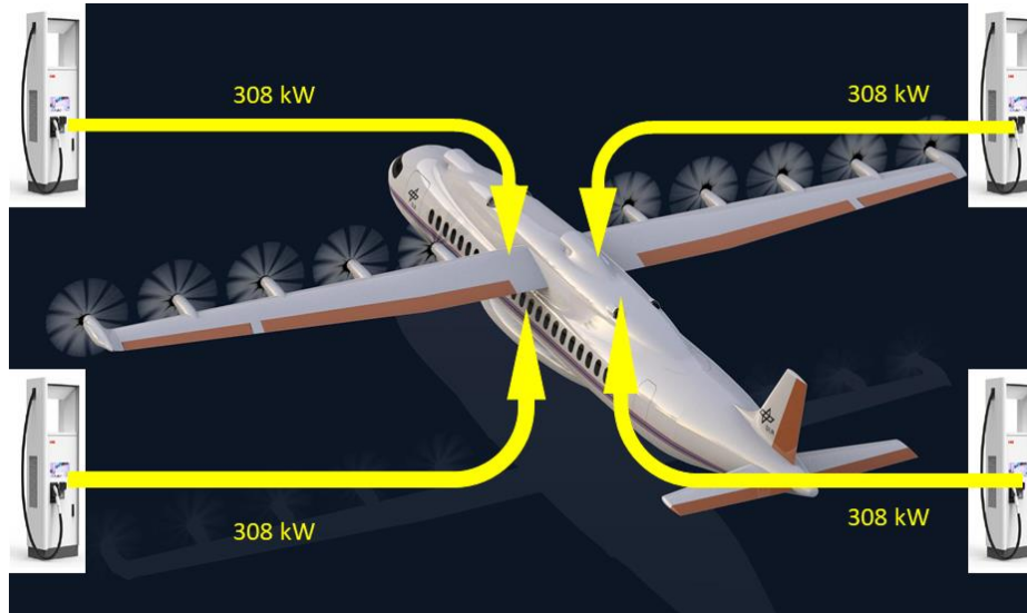
Figure 66. Fast Charging with two parallel stations per wing [124] [125]
