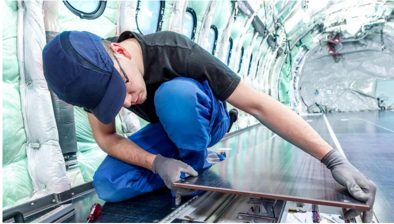
Figure 24 Installation of a sandwich aircraft floor panel [40]
